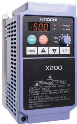
Traditional extract systems use a fan motor running at pole speed and adjust/calibrate the airflow at the fume cupboard via a manual volume control damper in the duct. With an inverter driven fan, the volume control damper is not needed (except where multiple branches exist). At commissioning the inverter is used to fine-tune the speed of the extract fan to achieve exactly the required face velocity.
